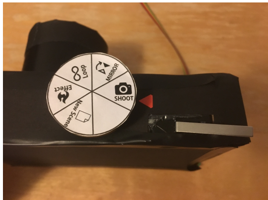
Figure 2. On top of the camera, potentiometer knob is located for users to switch between different modes of snapshot, mirror, loop, effect, and clear.
